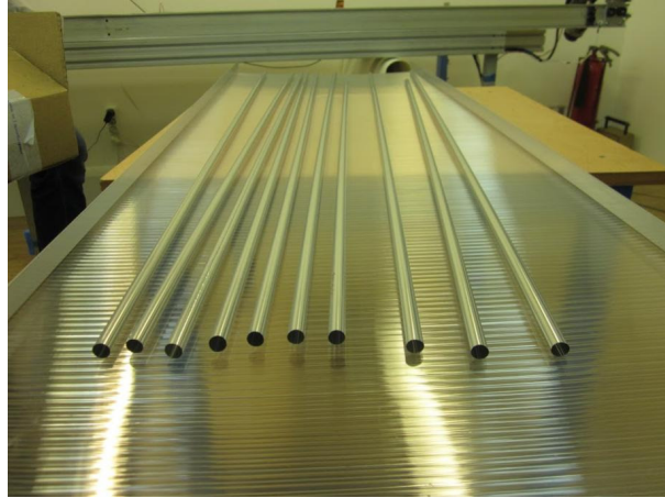
Рис. 7: Straw tubes of 20\ \mu wall thickness.
