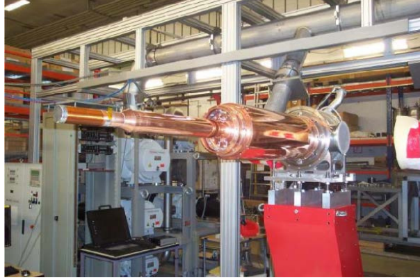
Рис. 1: The new dilution refrigerator for the Crystal Ball Frozen Spin Target.
