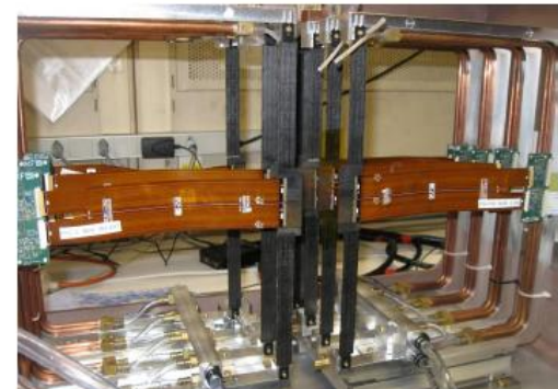
Small Acceptance Vertex Detector just before installation in 2016
