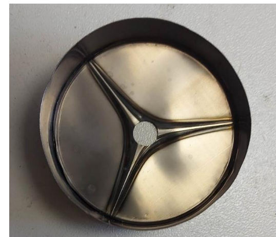
Screen with Ti foil after operation with SF 6 plasma
