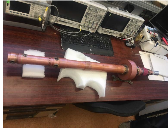
Gyrotron 28 GHz / 10 kW during bench test
