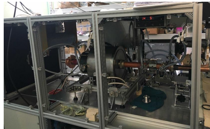
Gyrotron 28 GHz / 10 kW during bench test
