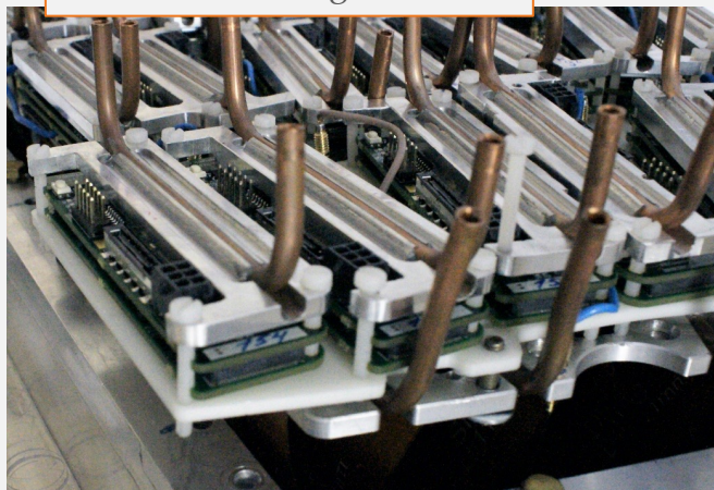
FECs with cooling radiators
