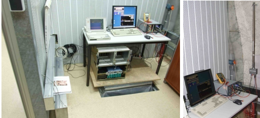
Fig. 9: Detectors developed at JINR for study of neutron background at EDELWEISS environment. Left picture is detector of fast neutrons; right one is detector of thermal neutrons (on the wall).
