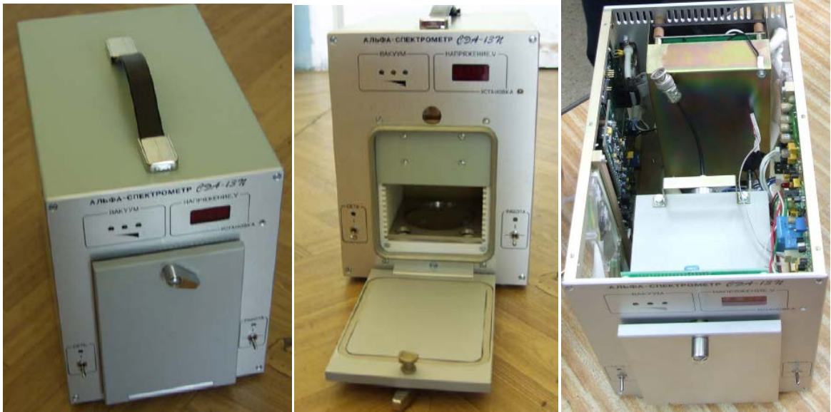
Fig. 14: Photo of the vacuum chamber of the alpha spectrometer containing electronic module (preamplifier, shaping amplifier, power supply, vacuum control module).
