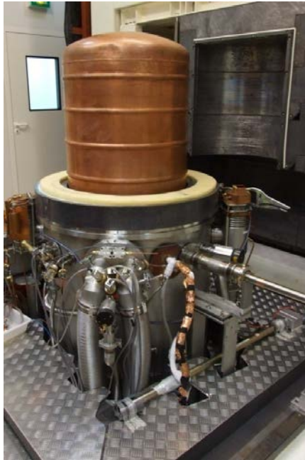
Fig. 10: Photo of the ^3\text{He} filled proportional counter installed at close proximity to the EDELWEISS cryostat.
