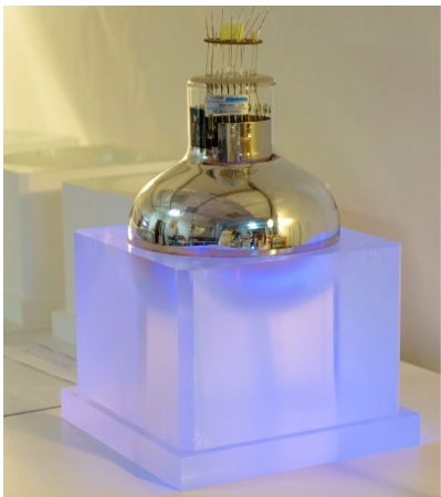
Figure 2. Left: one calorimeter Optical Module (OM), PS block equipped with a 8" PMT. Right: distribution of the energy resolution (FWHM) for the calorimeter Optical Modules with an average resolution of ~ 8 % FWHM for electrons 1 MeV, respectively.
