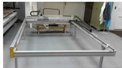
Fig. 18. Semi-automatic gluing system.
