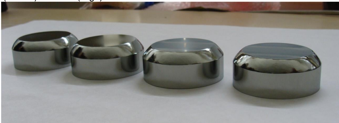
Figure 2. Photo of four HPGe point contact \nu\text{GeN} detectors.
