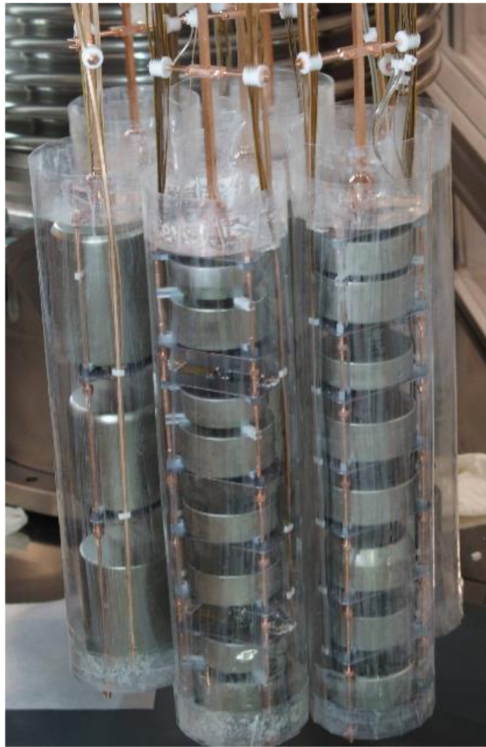
Fig. 4. Photo of GERDA Phase II detector array. Each of the seven strings is enclosed by a transparent mini-shroud.
