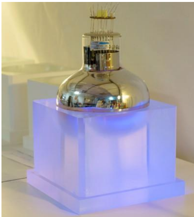
Figure 2. Left: one calorimeter Optical Module (OM), PS block equipped with a 8" PMT. Right: distribution of the energy resolution (FWHM) for the calorimeter Optical Modules with an average resolution of ~ 8 % FWHM for electrons 1 MeV, respectively.
