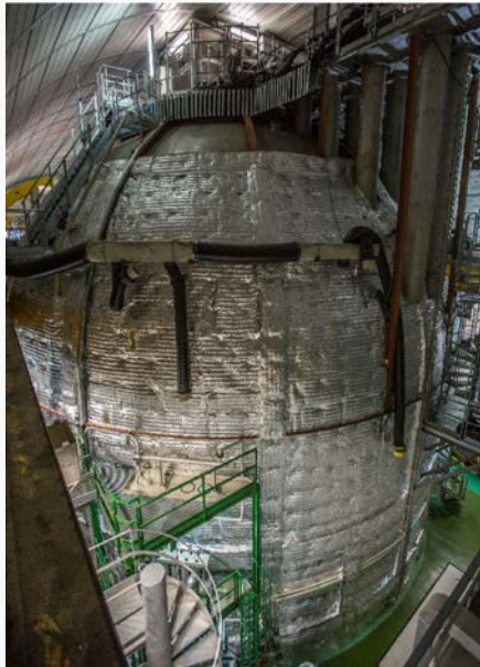
Figure 2 Photo of the detector insulated up to 14 m heights.
