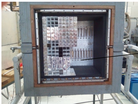
PHOS prototype (256 channels) installed in the electron test beam of the CERN PS (1-8 GeV beam).
