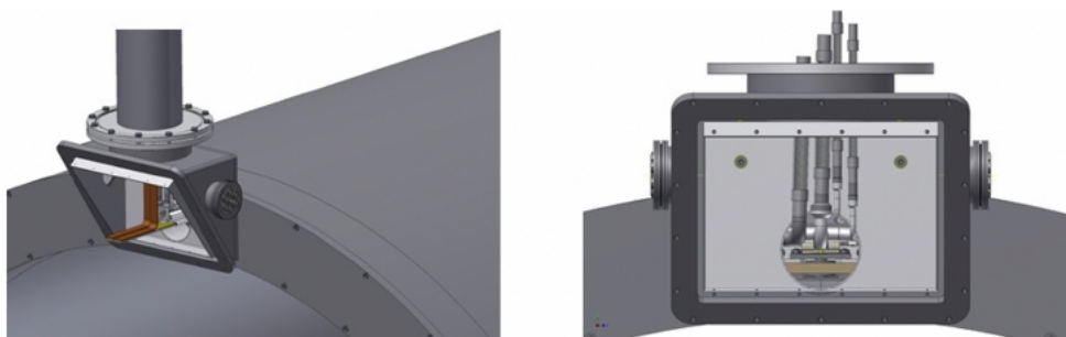
Figure 5.33: Connecting bus-bars and process pipes into the Interface box.
