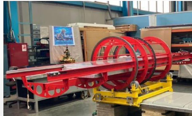
TOF installation bench in LHEP
