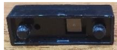
The real look of the SiPM PCB inserted to the housing
