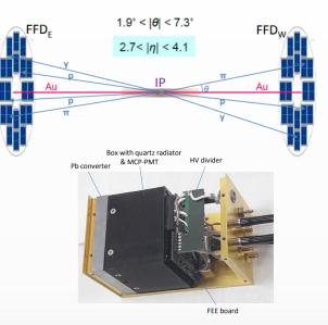
Cherenkov modules of FFDE and FFDW are available, mechanics of FFD sub-detectors is available for installation in container with vacuum beam tube
