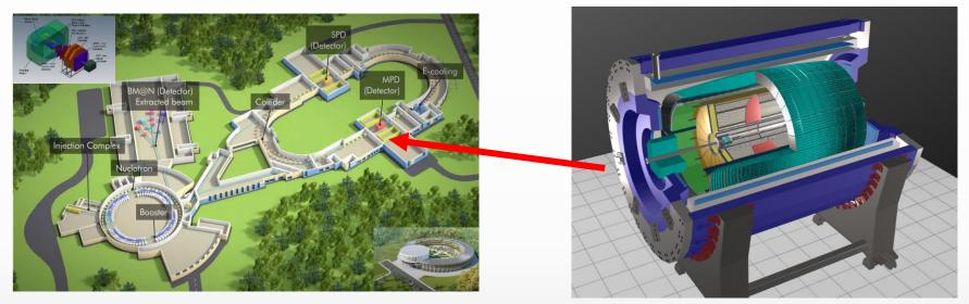
$\textbf{TPC:} \ |\Delta\phi| < 2\pi, \ |\eta| \le 1.6; \ \textbf{TOF, EMC:} \ |\Delta\phi| < 2\pi, \ |\eta| \le 1.4; \ \textbf{FFD:} \ |\Delta\phi| < 2\pi, \ 2.9 < |\eta| < 3.3; \ \textbf{FHCAL:} \ |\Delta\phi| < 2\pi, \ 2 < |\eta| < 5$
