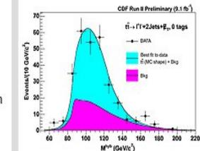
The plot shows the fit to the dilepton data sample. The data are the points with error bars. The background (purple) and the signal plus the background (cyan) for the reconstructed top quark mass are normalized to the numbers returned by the fit.
