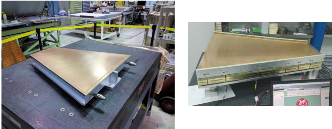
Figure A4.3: (left) pad plane bonded to Al strongback. (right) Complete prototype sector.
