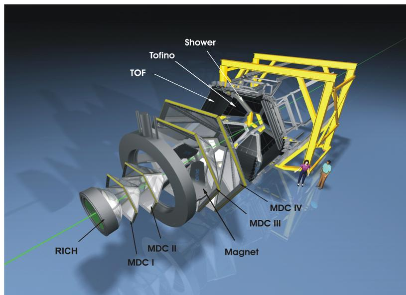
**Figure 2:** A schematic view of the HADES detector. Magnet is a superconducting toroid, MDC I-IV are the four planes of the multi-drift chambers, RICH is a Ring Imaging Cherenkov detector, Shower is a the pre-shower detector, TOF and TOFINO are the scintillation counters and Resistive Plate Chambers for time-of-flight measurements.
