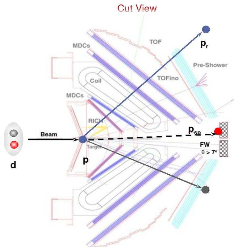
**Figure 3:** A schematic view of the HADES with FW during the experiment with deuteron beam. Spectator proton is detected by the FW.
