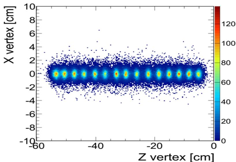
**Figure 5:** The reconstructed Z position of the segmented Au target (15 segments).
