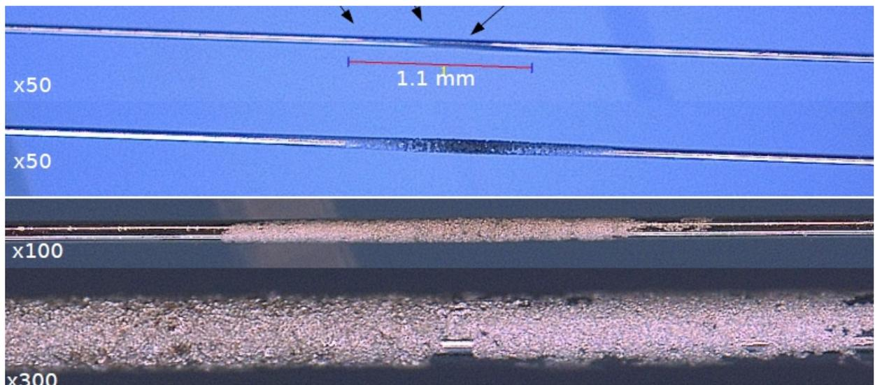
Figure 17: Single wire plane, showing dark deposits on field wires (diameter 80 $\mu$ m, Al) with different magnification factors using optical microscope.
