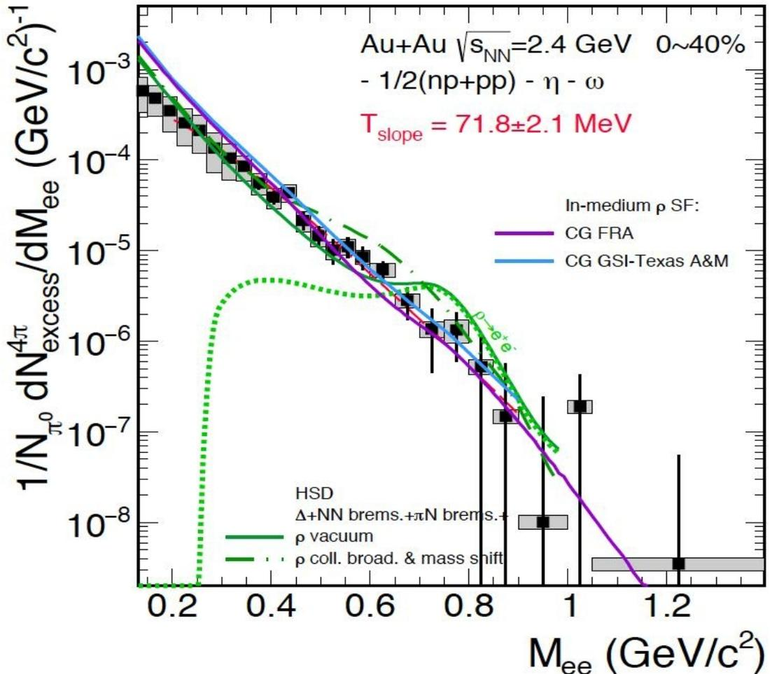
**Figure 9.** The di-electron yield for Au+Au reaction at 1.23 AGeV obtained with HADES. The solid lines are the cocktail calculations for different models without  $\eta$ - and  $\omega$ - mesons contribution. The dashed line is the contribution of the  $\rho$ -meson decay.
