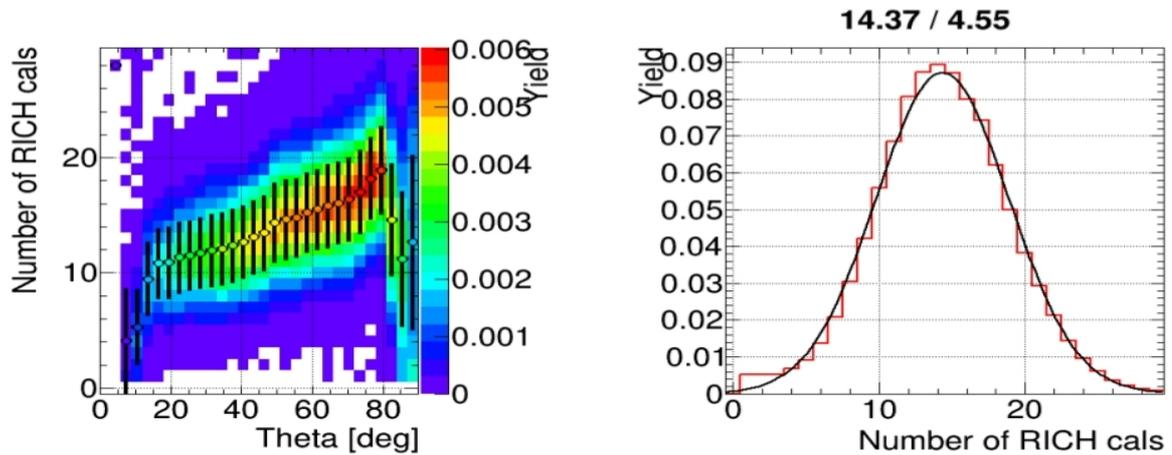
Figure 19: Results of the cherenkov ring reconstruction in new RICH. Left panel represents the dependence of the number of the fired pixels in photodetectors as a function of the electron emission angle. The right panel show the distribution of the number of the MAPMT fired pixels per electron ring.
