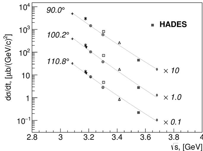
**Figure 16:** The energy dependence of the  $dp \rightarrow dp$  reaction cross section for the fixed angles in the cms. HADES measurements at 2.5 GeV are shown by the full squares. Lines correspond to the parameterization  $s^{-16}$  coming from the constituent counting rules [24].
