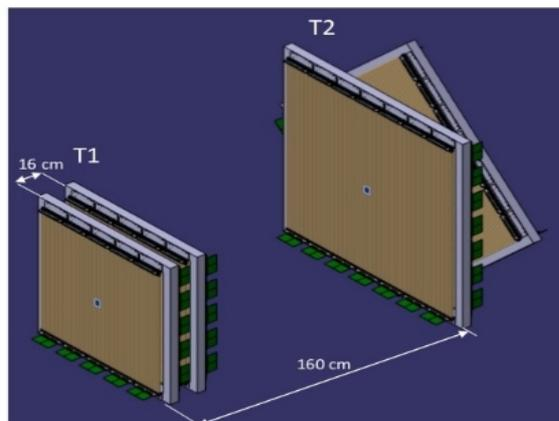
Figure 20: Schematic view of the Forward Detector based on the PANDA straw tubes.
