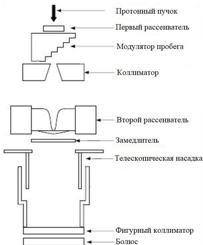
Fig. 1. Scheme of the treatment beam shaping in the treatment room.
