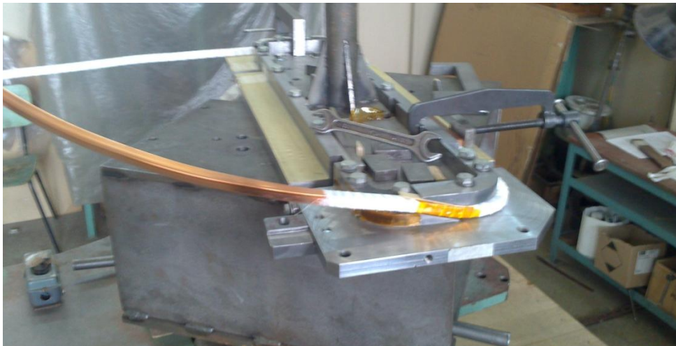
Winding process of coils of the toroid section
