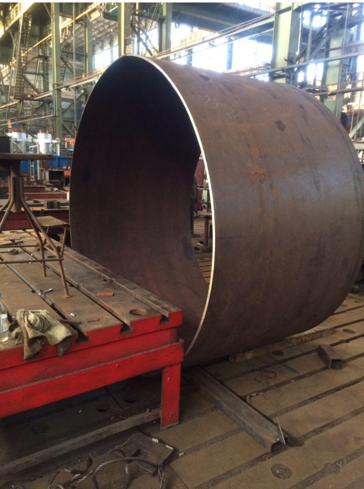
Central part of high voltage vessel in Novosibirsk workshop
