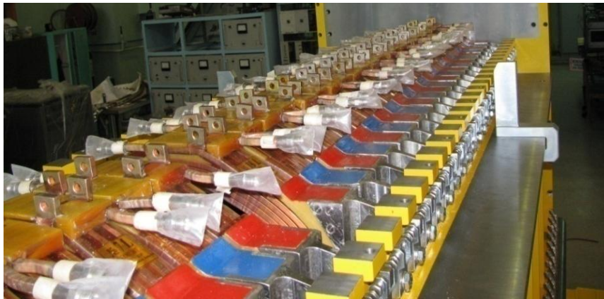
“Left” and “Right” coils like COSY design. The idea is decreasing role of the magnetic field induced by wire splice
