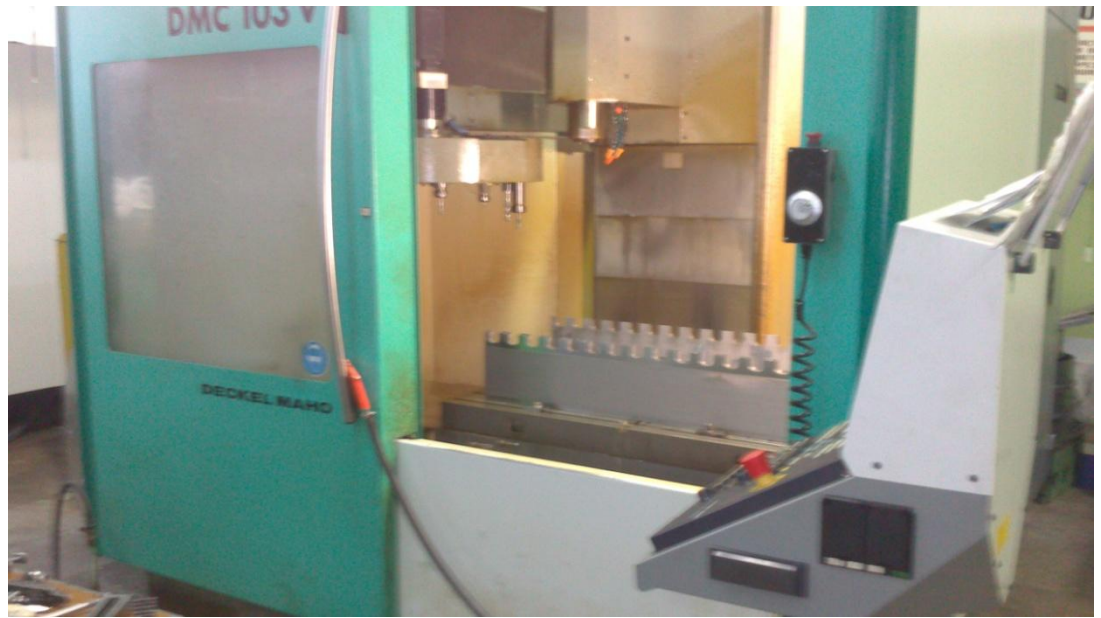
Cover of section is installed on numerically controlled machine tool
