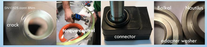
**Glass cracking tests showed:** for <u>the same</u> quality of grinding surfaces around the holes old spheres withstand tightening torque of the connector up to15 Nm without cracking, while the new ones begin to crack at 6 Nm (30% holes cracked at 15 Nm).
