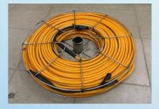
**OM cable** - most common cable of Baikal-GVD Connects **OM** with **CM**, is part of the spectrometric channel Includes coaxial pair, power supply, slow communication line Has 2 hermetic connectors, 2 hermetic sleeves, length 90 m
