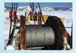
**String carrier** - stainless steel armored geophysical cable The bottom part of the buoy rope of a length ~700 m Consist of the core with 7 electrical lines and 2 armoring layers of stainless steel wires Diameter 9.3 mm, breaking load 43 kN
