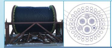
Hybrid optical-electrical carrier cable with plastic sheath 3 single-mode optic fibers in stainless tube (x2) 3+1 electric lines of total section ~16 mm<sup>2</sup> Working load to 18kN, breaking load 65 kN Diameter 19.2 mm, length ~6,5 km
