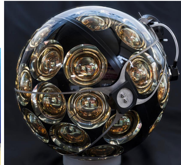
31 3" PMTs in glass sphere Multi-PMT DOM
