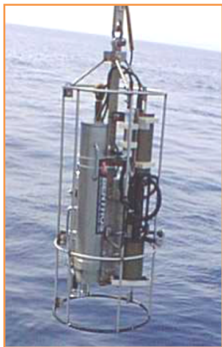
Ligh transmission (absorption, attenuation) vs depth
