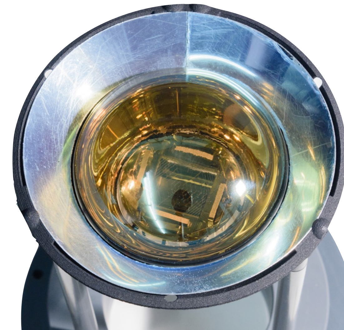
Reflector with PMT in test support structure
