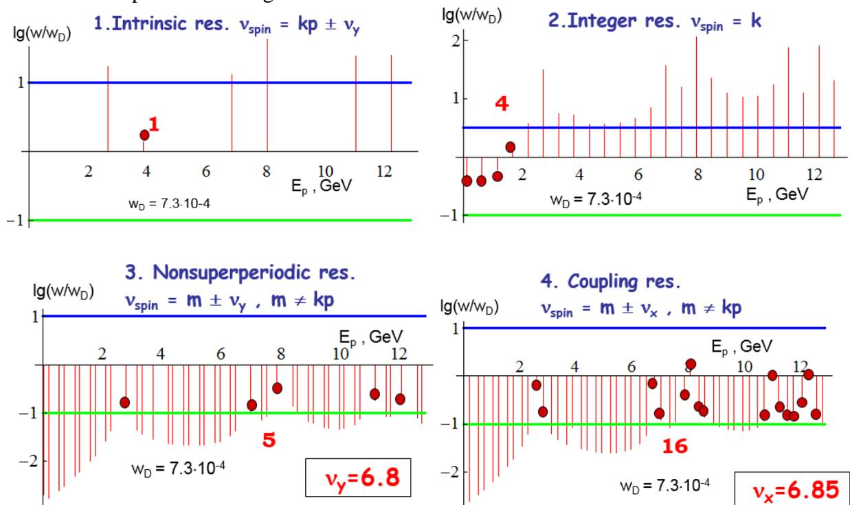
Fig. 7. Linear spin resonances in the Nuclotron at polarized proton mode.
