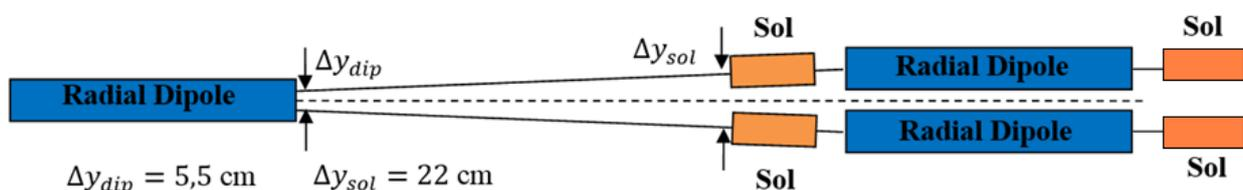
Fig. 4. Placement of weak control solenoids in vertical plane together with radial dipoles.
