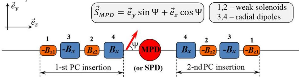
Fig. 2. Detail scheme of the PC's insertions in the collider in the ST regime.
