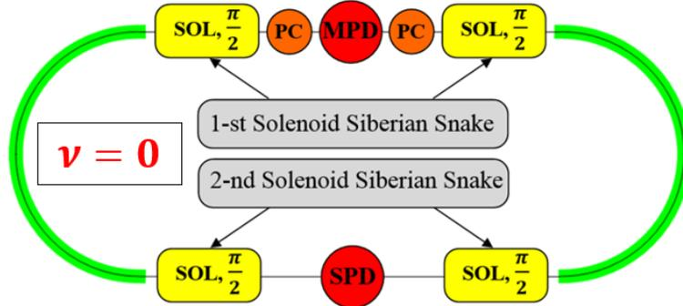
Fig. 5. Scheme of realization ST regime in NICA Collider.
