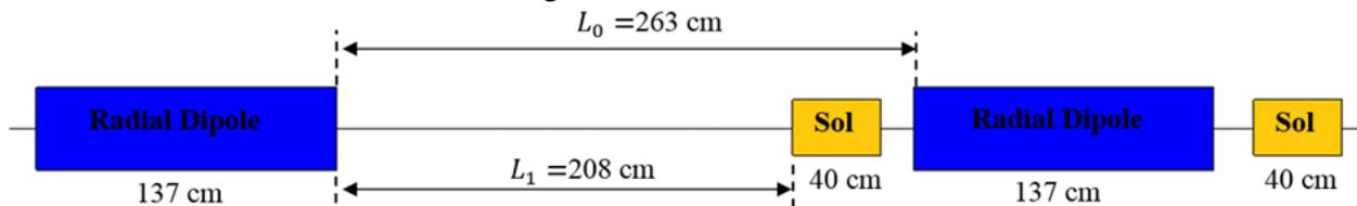
Fig. 3. Placement of weak control solenoids in horizontal plane.
