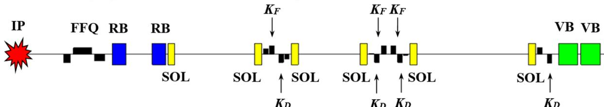
Fig.6. Distributed snake (one half) based on short 6T SC solenoids.
