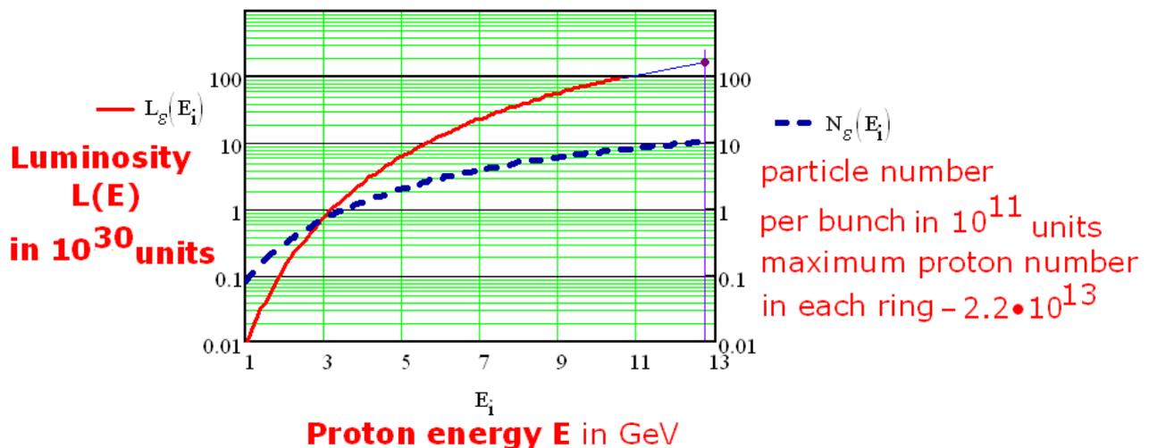
Fig. 2.1. Normalized dependence of pp-collision luminosity on proton kinetic energy.
