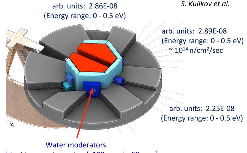
(ambient temperature, size d=120 mm, h=60 mm)
