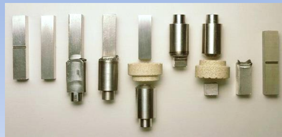
... arc stud welding (ASW)
