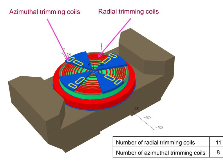
Checking of magnetic field direction between trimming coils was carried out during Launching and Tuning Works
