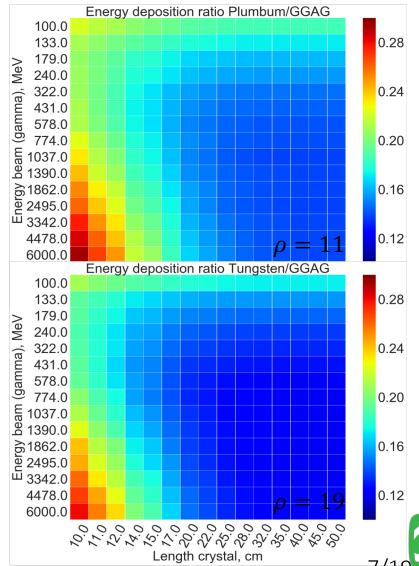
At greater lengths and energies, about 80% –85% of the energy dep is lost, since the ratios of a pure crystal to a crystal with a coating are 1 mm<sup>2</sup> to 8 mm<sup>2</sup>
