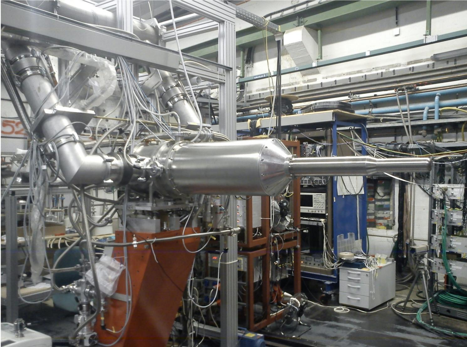
**Dubna-Mainz Frozen Spin Target** (available since 05.2010). For the double polarization measurements planned with the Crystal Ball detector on polarized protons and deuterons a specially designed, large horizontal  $^3\text{He}/^4\text{He}$  dilution refrigerator has been built in cooperation with the Joint Institute for Nuclear Research. Superconducting holding magnet permits longitudinal and transverse polarizations. Butanol and trityl doped deuterated butanol are used in experiments.
