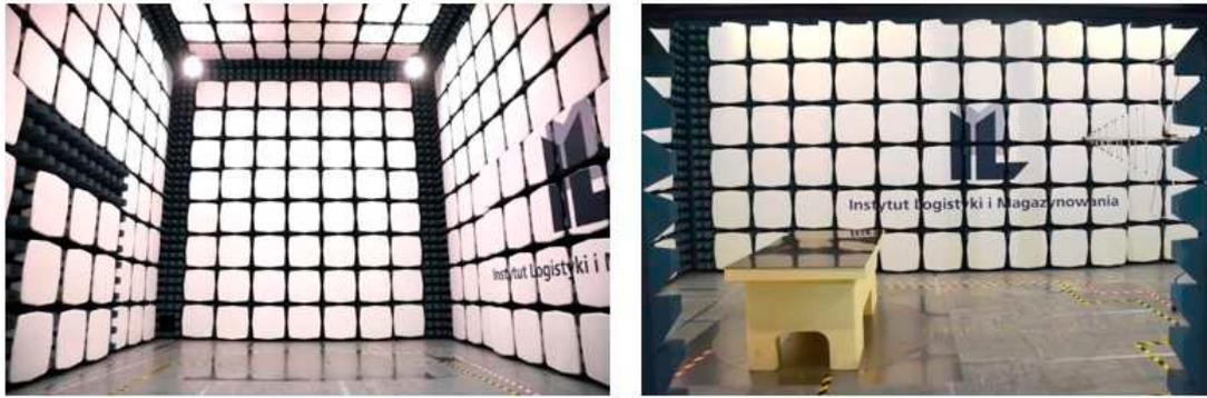
**Figure 2: Semi-anechoic chamber in Laboratory of Electronic Devices of the Institute of Logistics and Warehousing.**
