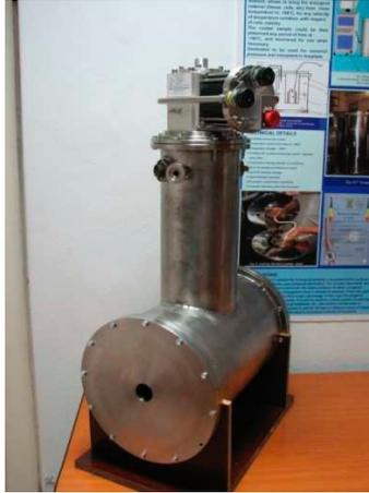
Figure 3: The cryostat and cooling cryogenic system.
