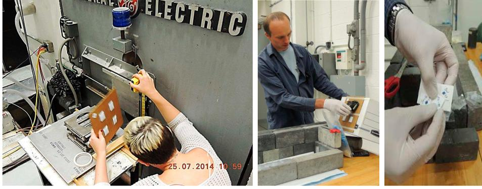
Figure 3: Foils positioning, dose measurement and uncovering
