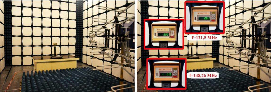
Figure 5: Left - an example of electromagnetic field immunity test of the electronic scale in semi-anechoic chamber, right - the impact of radiated RF electromagnetic field on the operation of the electronic scale.
