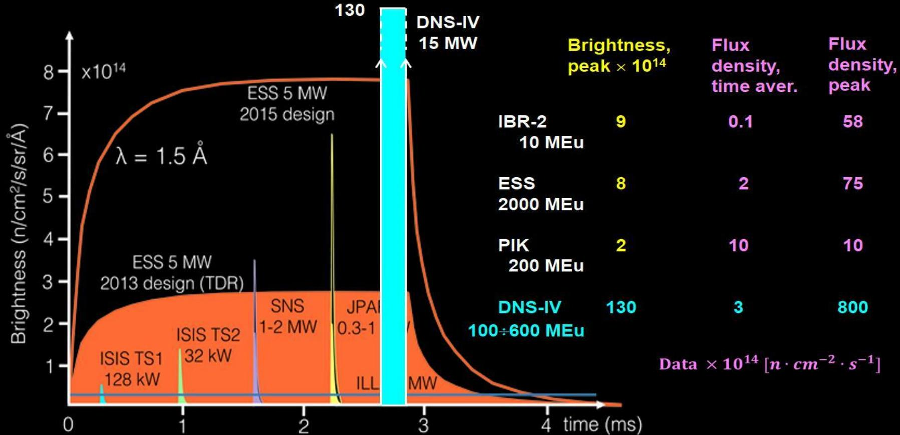
Single-pulse source brightness as a function of time at wavelength of 1.5 Å at ESS, ILL, SNS, J-PARC and ISIS Target Stations 1 and 2. In each case, the thermal moderator with the highest peak brightness shown. (Source: ESS)
