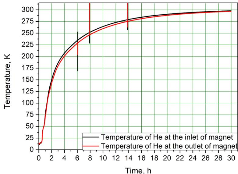
**Cooling-down (left) and warm-up (right) of the quadrupole doublet for the NICA booster. Black line is inlet and red line – outlet of the magnet.**
