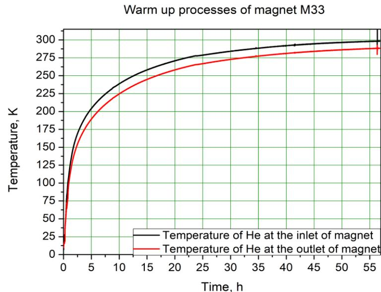
**Cooling-down (left) and warm-up (right) of the dipole magnet for the NICA booster. Black line is inlet and red line – outlet of the magnet.**
