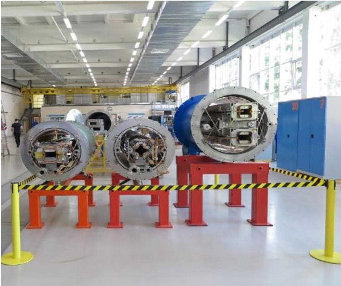
Series dipole magnet (left) and doublet (center) for NICA booster, and first of series dipole magnet for NICA collider (right).
