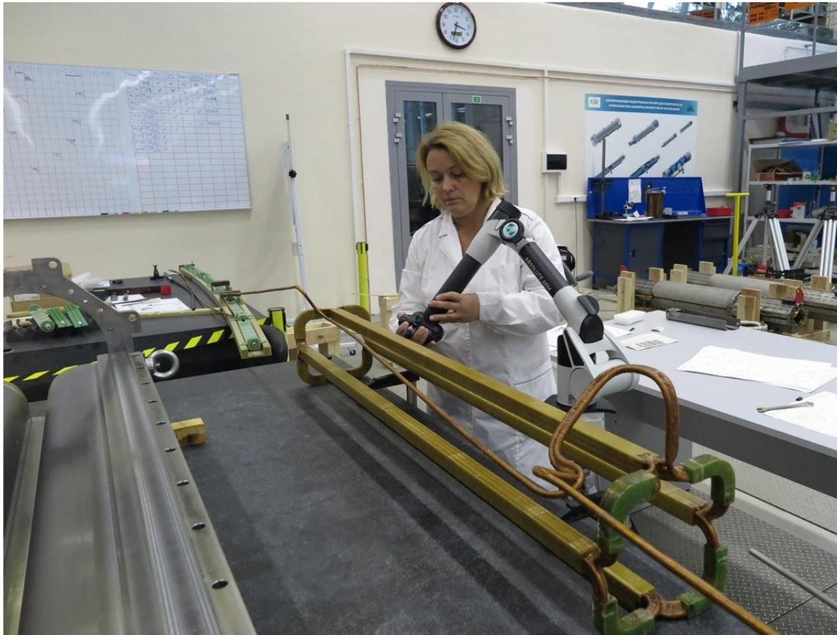
Check and assembly of the yoke and the coil for the SIS100 quadrupole magnet
