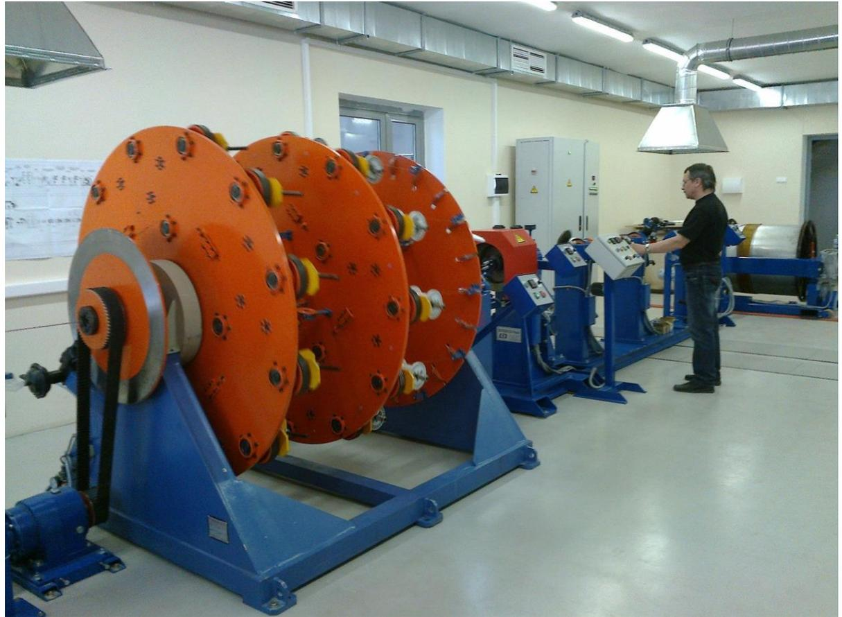
Machine for production Nuclotron-type superconducting cable
