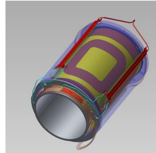
**The coil for the NICA booster corrector magnet manufacturing**
