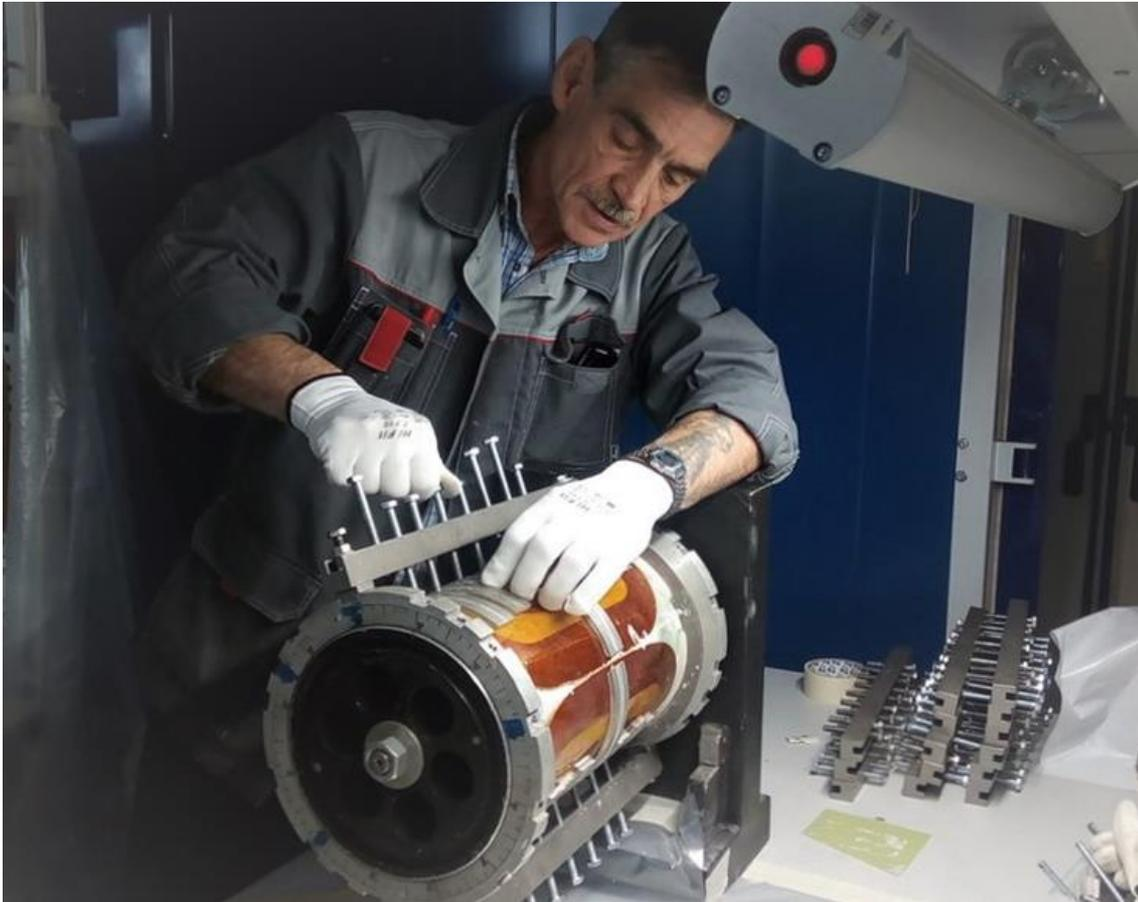
24 steering magnets will have two coils each (horizontal and vertical dipole coils) and 8 corrector magnets will contain four coils each (normal and screw sextupole, screw quadrupole and octupole coils).
