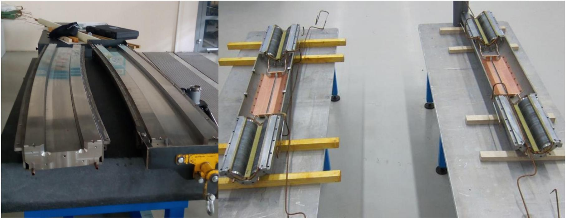
**Half-coils assembling with half-yokes for the booster dipole magnet (left) and doublet of the lenses (right)**
