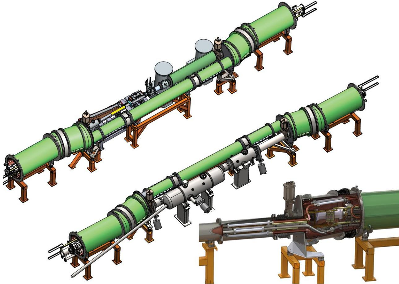
There are two bypass lines for injection and extraction of the beam. Vacuum shells and thermal shields are in the manufacturing stage, SC bus bars and helium collectors are in the design stage.
