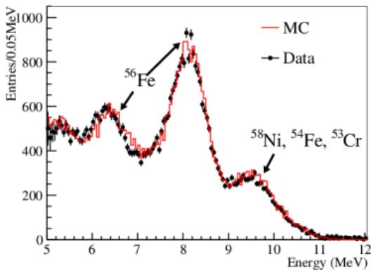
**Figure:** Energy spectrum of the events near the top of ADs in the Far Hall.
