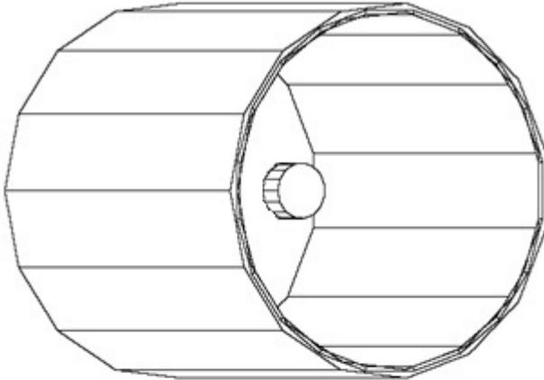
The hodoscope array consists of 20 independent BC-408 plastic scintillator staves arranged to form a complete cylinder 653.8 mm long with a 129 mm radius and 4.0 mm thickness.
