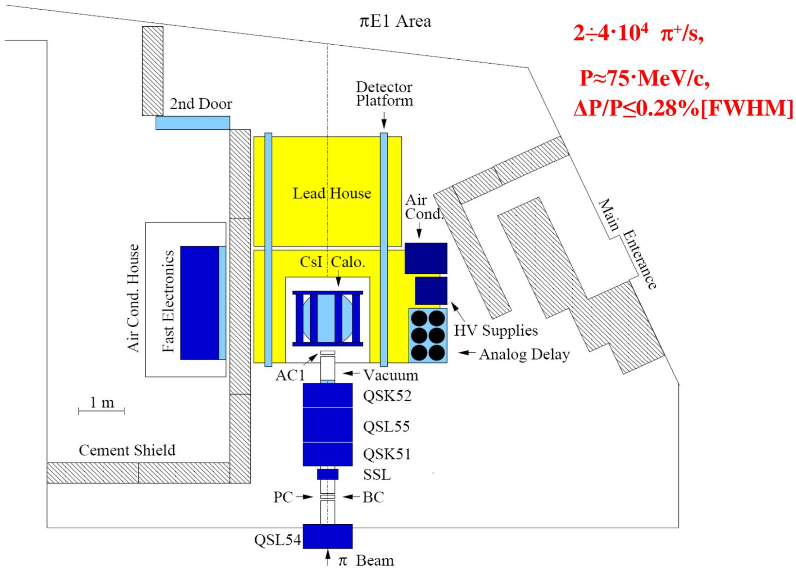
**A layout of the PSI  $\pi E1$  experimental area for the PEN experiment (top view)**
