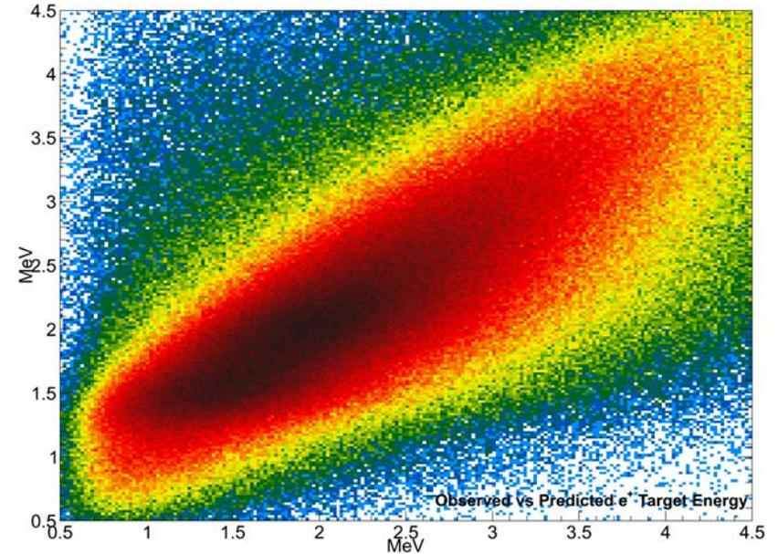
Observed energies are obtained from the target waveform and predicted energies are obtained from mTPC, MWPC, and beam counters for the pion and positron.
