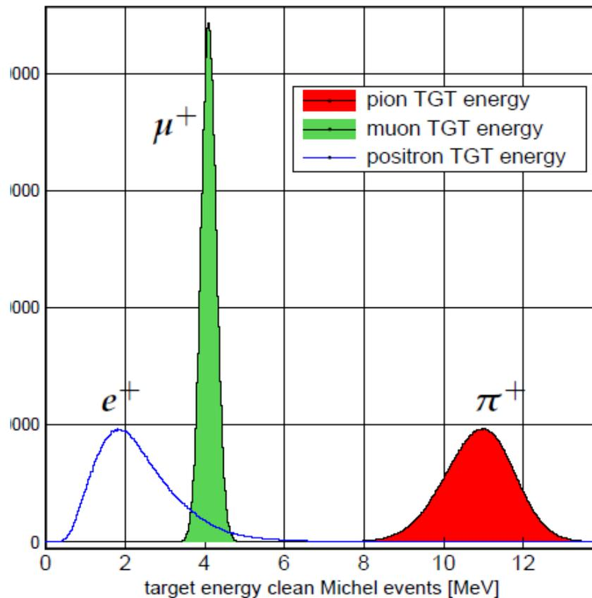
Target waveform analysis for  $\pi \rightarrow \mu \rightarrow e$  decay chains in which the three signals are well separated. Removal of the predicted pion and positron signals leaves a clean 4MeV muon signal.
