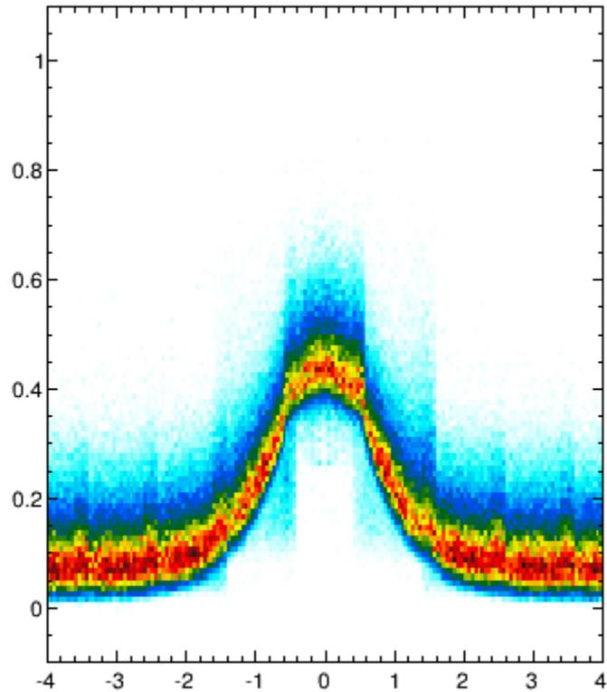
induced charge fraction vs strip distance simulation
