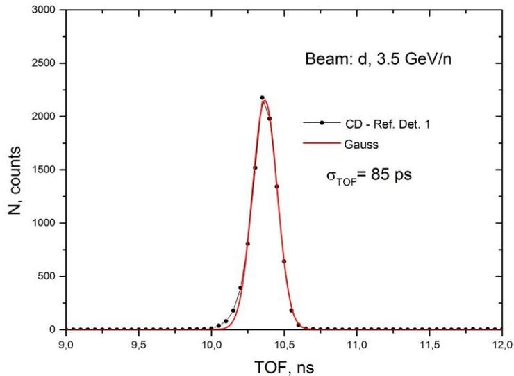
The time resolution of CD detector measured with standalone readout electronics is:
