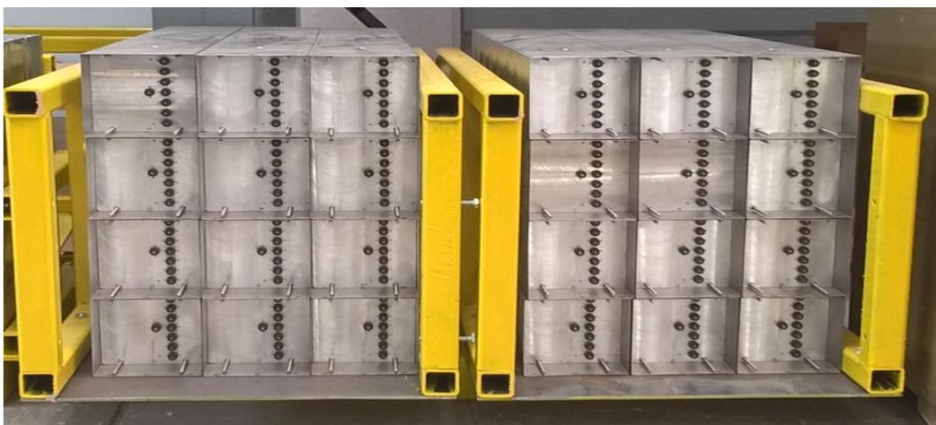
According to the agreement with INR RAS about 80% of FHCAL modules are already produced and tested with cosmic muons.
