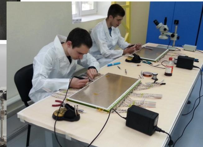
Cables and connectors soldering
