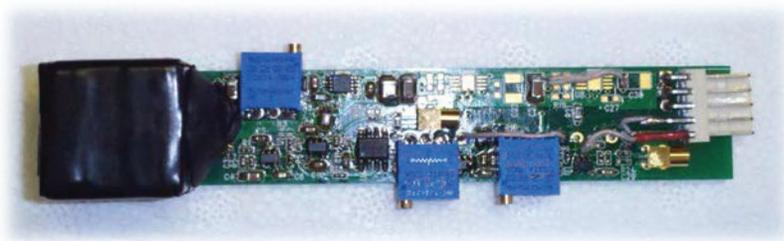
**Figure 2.** Trigger counter based on SiPM SensL.
