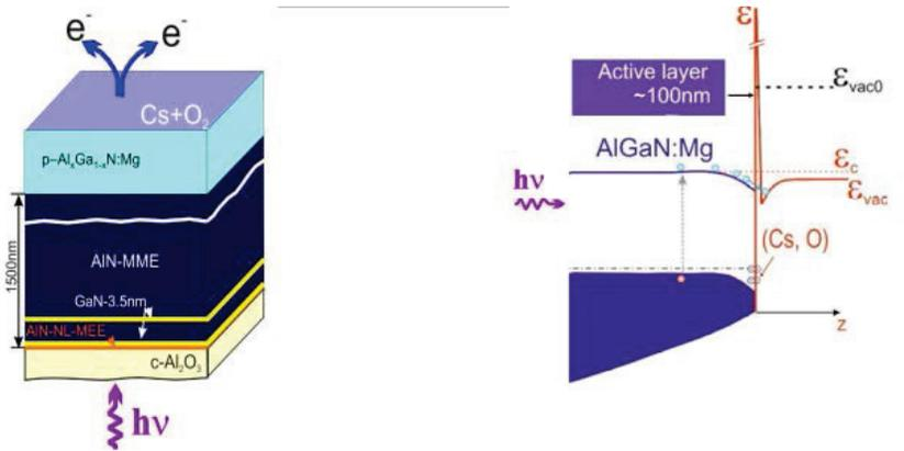
Fig.1. After manufacturing UV-photocathode heterostructure is activated with Cs/O<sub>2</sub> to get negative electron affinity.
