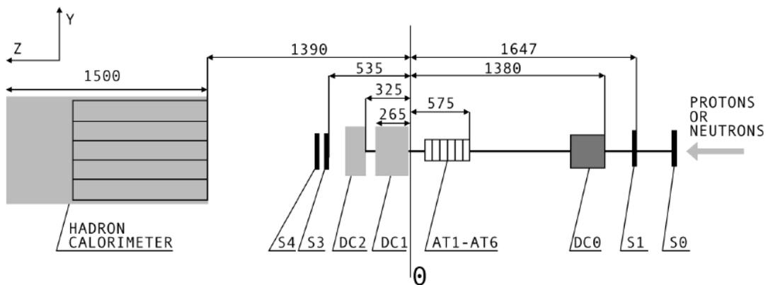
Fig. 11. Side view scheme of the ALPOM2 set up positioned on the secondary proton/neutron beam line, including scintillation counters (S0, S1, S3, S4); drift chambers (DC0, DC1, DC2); hadron calorimeter. The analyzing materials of the polarimeter were located between DC0 and DC1. Here a CH active target (AT1 -AT6), is shown as an example. Dimensions are in mm.
