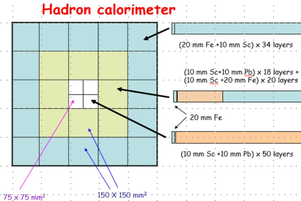
FIG. 13: Design of the different bars of the hadron sampling calorimeter used in the ALPOM2 setup.
