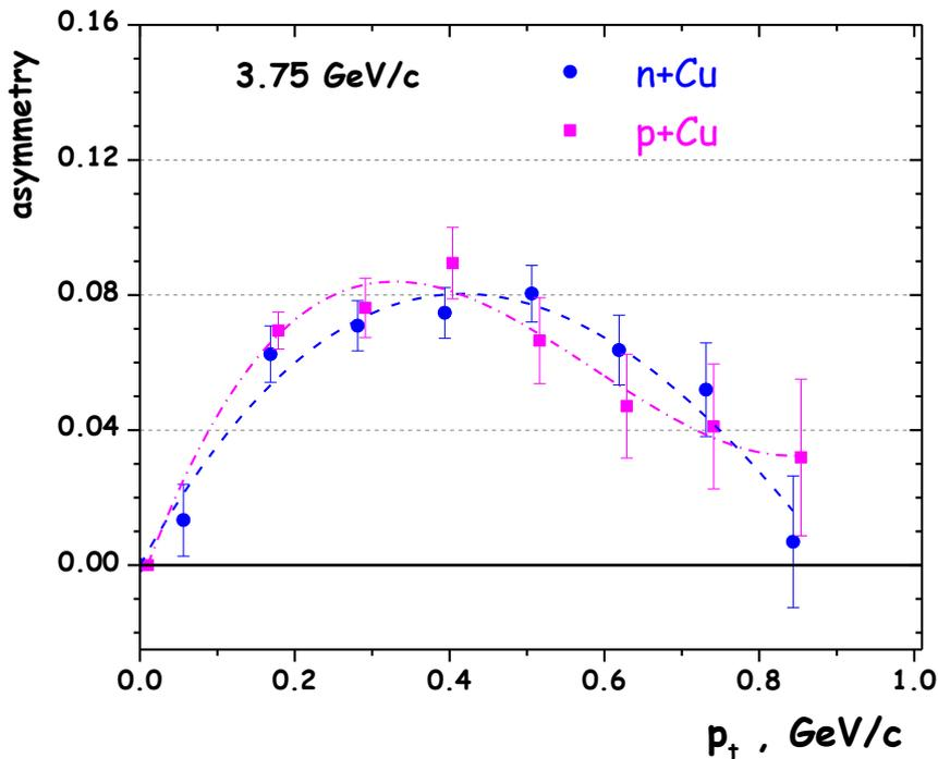
Fig.21. The asymmetry vs transfer momentum for neutron and proton scattering on Cu-target at 3.75 GeV/c.
