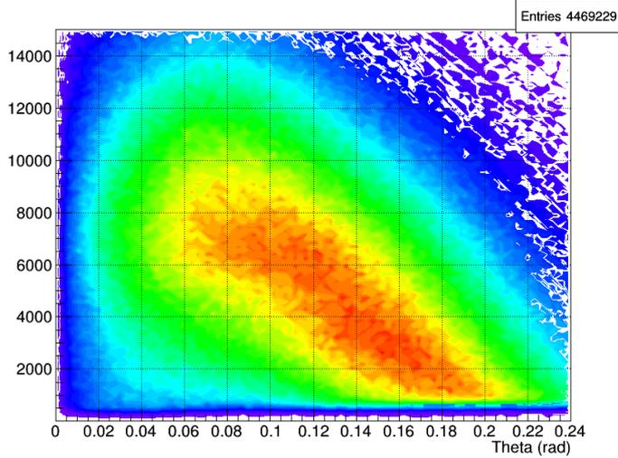
Fig.15. The energy deposit vs scattering angle for neutrons of 3.75 GeV/c on C target.
