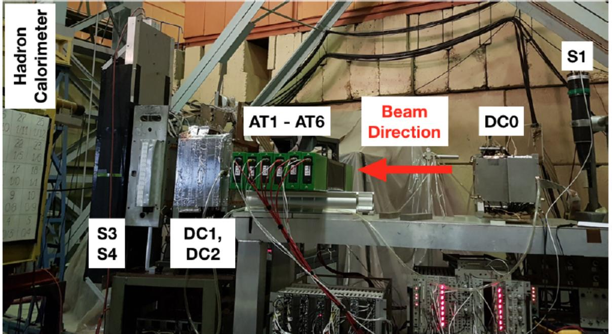
FIG. 12: Photograph of the ALPOM2 set up with the CH active target analyzer, which was used for a subset of neutron polarimetry measurements, in place.
