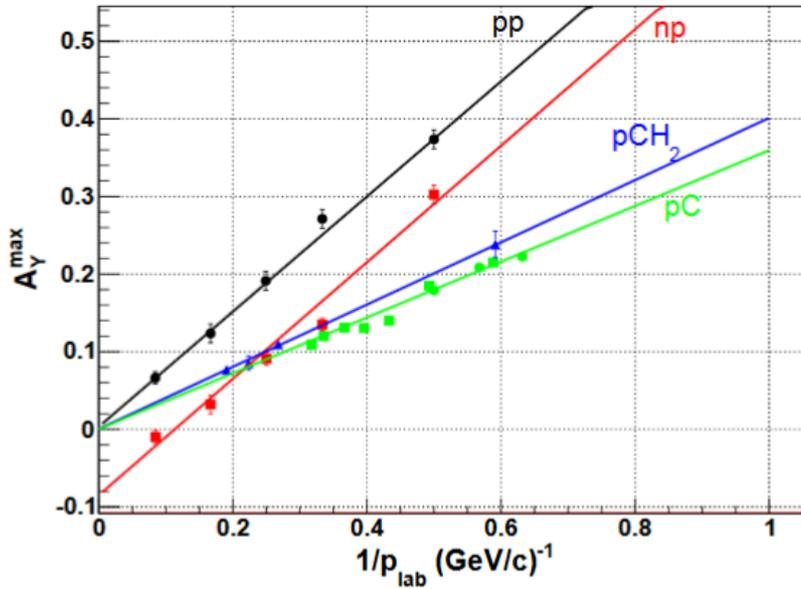
Fig. 3: The dependence of the maximum of  $A_Y$  on  $1/p_{\text{lab}}$ . Black circles: ANL  $d(p,p)n$  data [29, 30]; black line: linear fit. Red squares: ANL  $d(p,n)p$  data [29, 30]; red line: linear fit. Blue triangles [25]:  $p + \text{CH}_2 \rightarrow \text{charged} + X$ ; blue line: linear fit [25]. Green squares [31] and circles [32]:  $p + \text{C} \rightarrow \text{charged} + X$ ; green line: linear fit [25].
