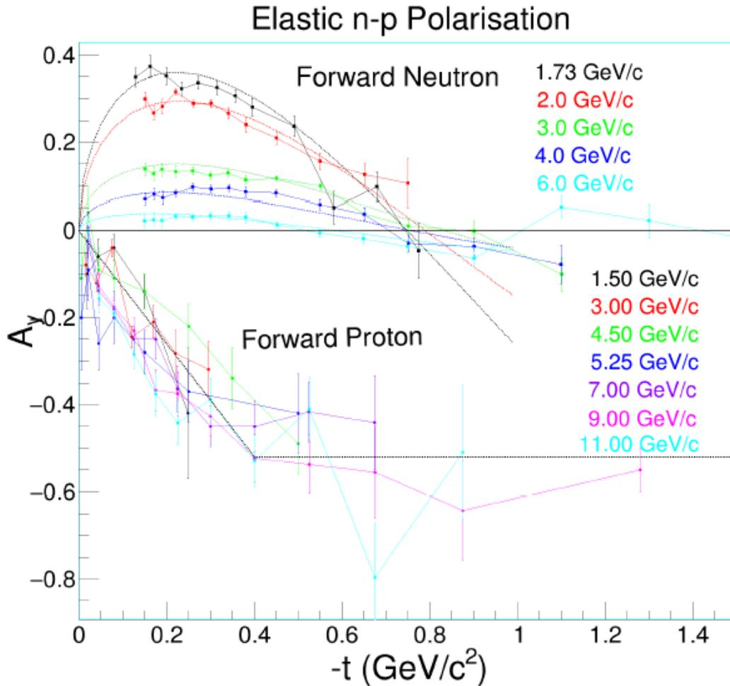
Fig. 4: Top: the  $p_{\text{lab}}$  and  $t$ -dependence of the analyzing power of elastic pn scattering [29, 30]. The smooth dotted lines show the fit of Ref. [33] to the pn data. Bottom: the  $p_{\text{lab}}$  and  $t$  dependence of charge-exchange np scattering [34, 35]. The color-coding relates the data to momentum labels.
