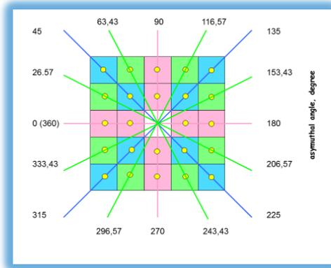
Fig.17. Azimuthal segmentation of the hadron calorimeter for the asymmetry measurements.
