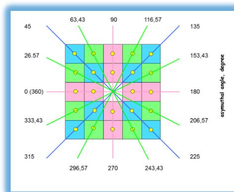
Fig. 14: Azimuthal segmentation available from the hadron calorimeter for asymmetry measurements.
