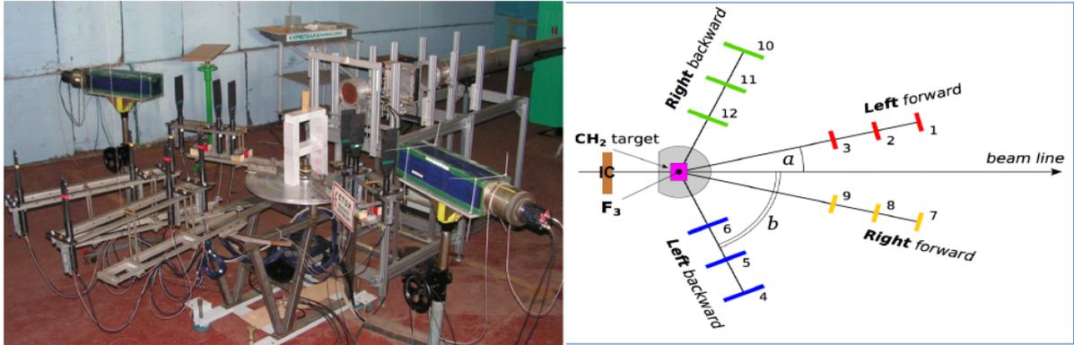
FIG. 5: The F3 polarimeter. IC is an ionization chamber. The F3 left, right forward and backward arms have three scintillation counters at angles  $a$  and  $b$  with respect to the beam-line.
