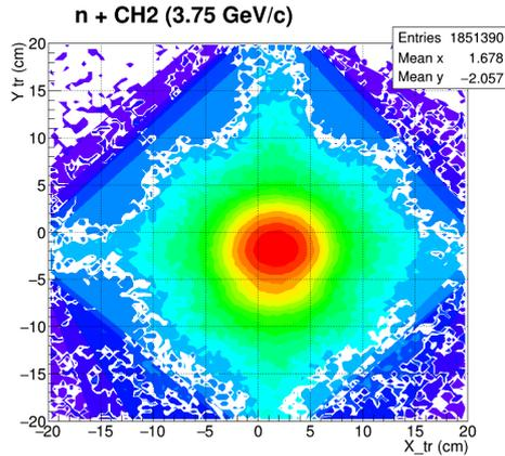
Fig.10. Position of neutron beam at the CH2 target.
