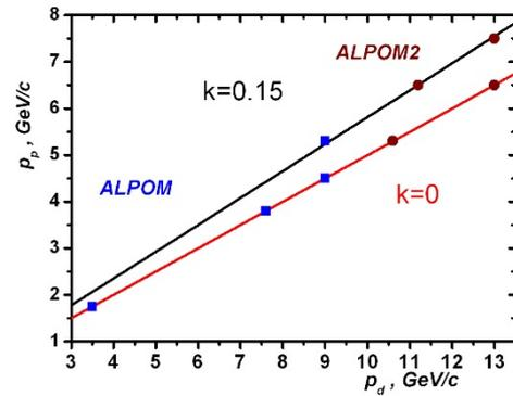
Fig. 9 Dependence of proton momentum at which the proton polarization is equal to the deuteron polarization ( $k=0.15$ ) versus the primary deuteron momentum. Blue points: old measurements; red points: future measurements.
