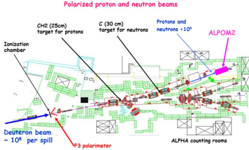
Fig. 7. Scheme of transportation polarized beams from Nuclotron to the ALPOM2 setup and the location of F3 polarimeter and production target for proton and neutron beams
