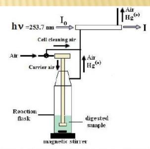
Schematic diagram of the "home-made cold-vapor system" used for atomization and volatilization of mercury
