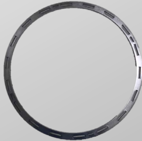
Silicon rings with lower background contribution instead of copper ones
