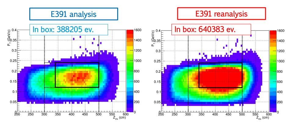
Total BG: the same level Acceptance : increased on 65% (In comparison with E391 final result)
