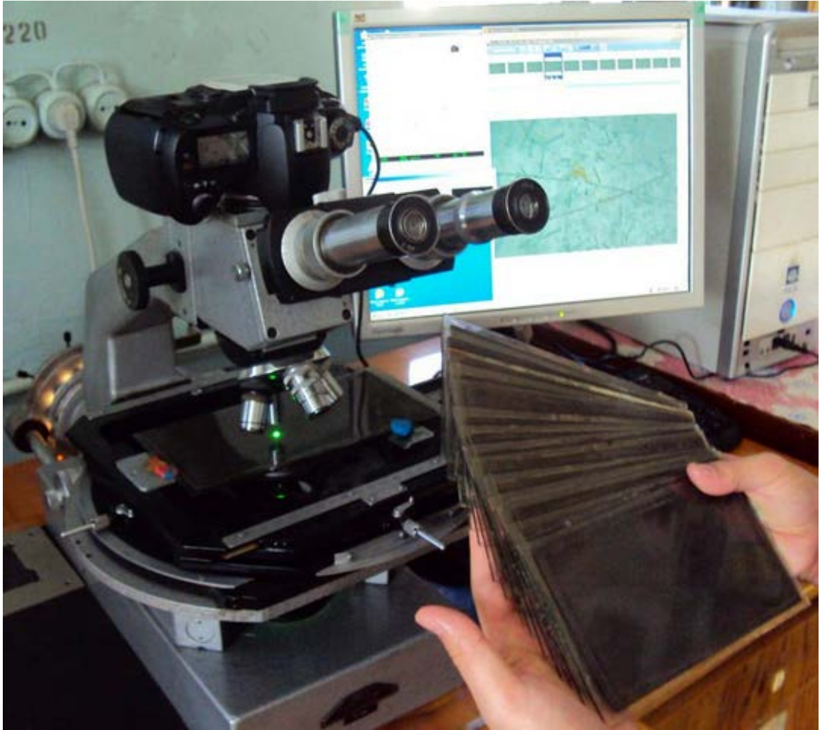
Fig. 3. Developed 500 \mu\text{m} NTE pellicles glued on glass support. Beam nuclei entered through edge along long side.
