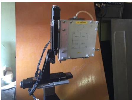
Fig.4. Freon beam chamber in HILUM-2 experiment at U-70 (Protvino).
