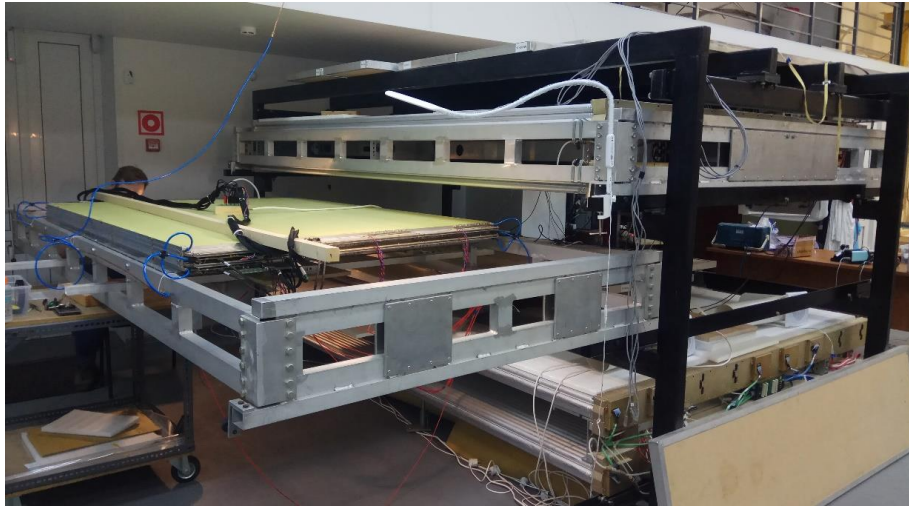
Fig. 15. Quadruplet preparation for the functionality test at the cosmic ray bench.
