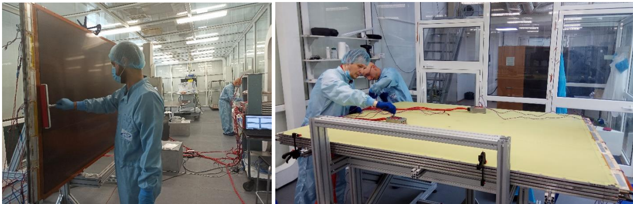
Fig. 14. Quadruplet assembly procedure in the clean room.
