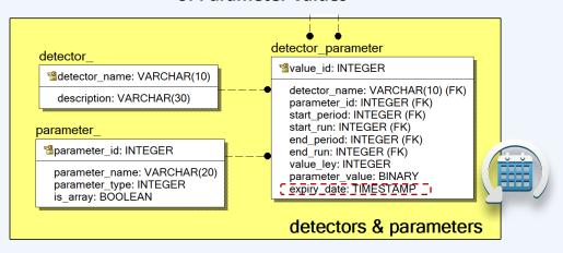
Parameter values need to be retained in case of updating. When parameter values are updated, the database saves the replaced data with the current expiry date.
