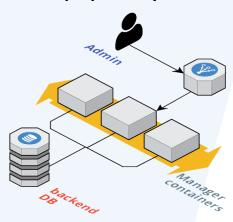
The common Configuration and Deployment System is planned to be based on Docker containers and shell scripts
