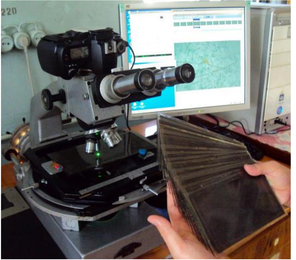
Fig. 3. Developed 500 \mu\text{m} NTE pellicles glued on glass support. Beam nuclei entered through edge along long side.
