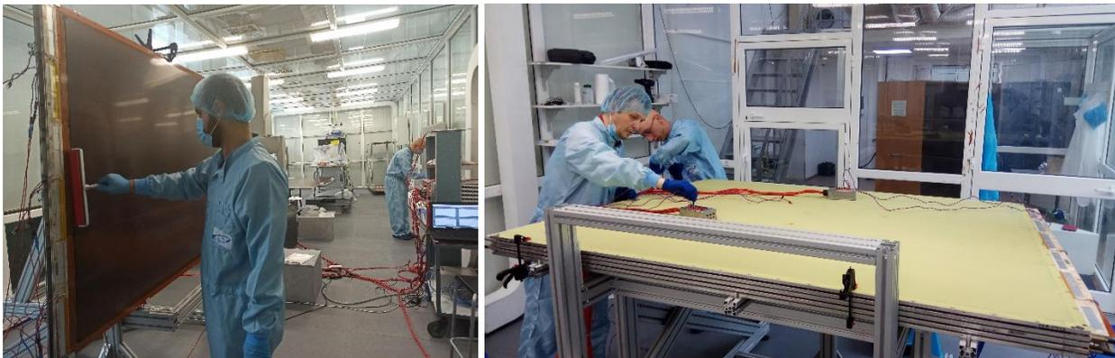
**Fig. 14.** Quadruplet assembly procedure in the clean room.
