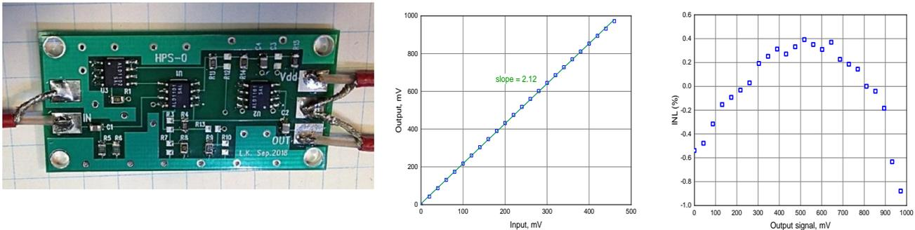
**Fig.3.** HEC shaper prototype and the non-linearity measurements.
