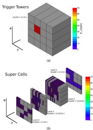
**Fig.1.** An electron (with 70 GeV of transverse energy) as seen by the existing Level-1 Calorimeter trigger electronics (a) and by the proposed upgraded trigger electronics (b).
