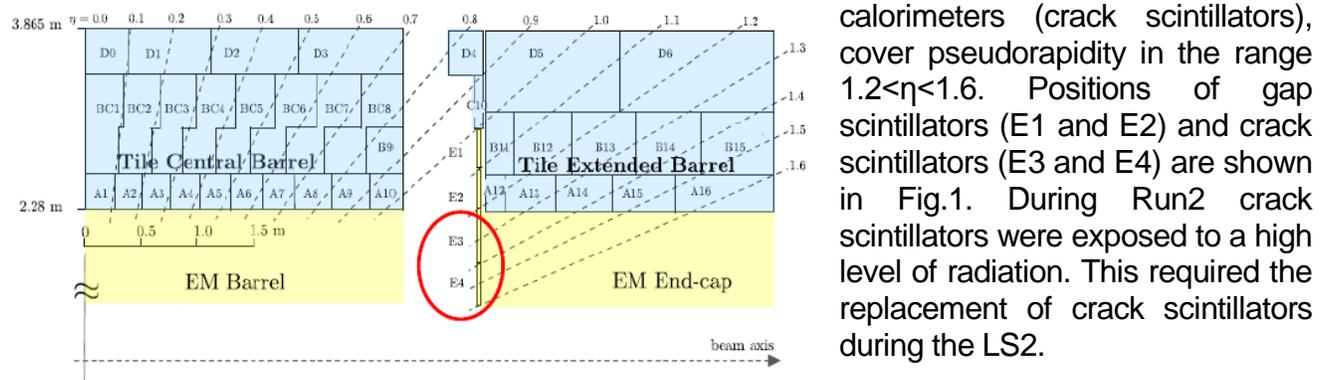
**Fig.5.** Position of gap and crack scintillators. Crack scintillators E3 and E4 position highlighted in red.
