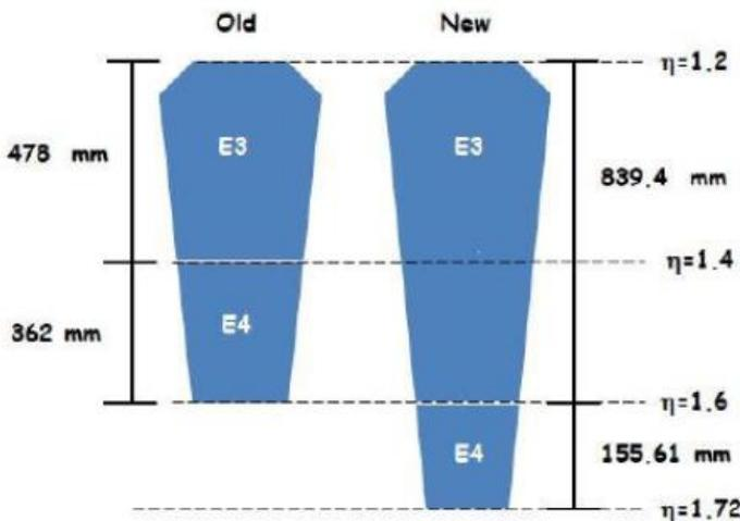
In order to increase the electron reconstruction efficiency in the EM calorimeter region it was decided to increase the length of the E3+E4 module. The new geometry of the crack scintillators is presented in Fig. 6. New E3+E4 module covers a region  $1.2 < \eta < 1.72$ .
