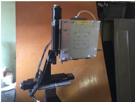
In the HILUM-2 experiment at Protvino we study performance of the mini-modules of the ATLAS LAr calorimeters with high-intensity proton beams at U-70. The goal is to investigate the influence of the space charge built in thin LAr gap on the shape of the calorimeter signal. We have designed and produced the beam chamber (Fig. 4) and corresponding electronics for the beam profile monitoring.
