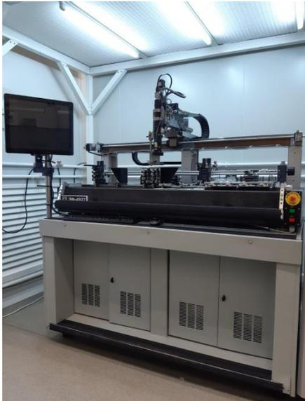
**Ladder Assembly Device** and corresponding fixtures were developed and produced for the assembly of the BM@N and CBM ladders. Accuracy of the sensor positioning is tested.
