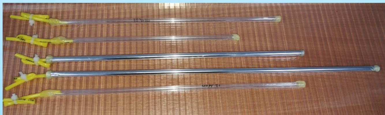
Samples of straw tubes pressurized at 3-4 bar
