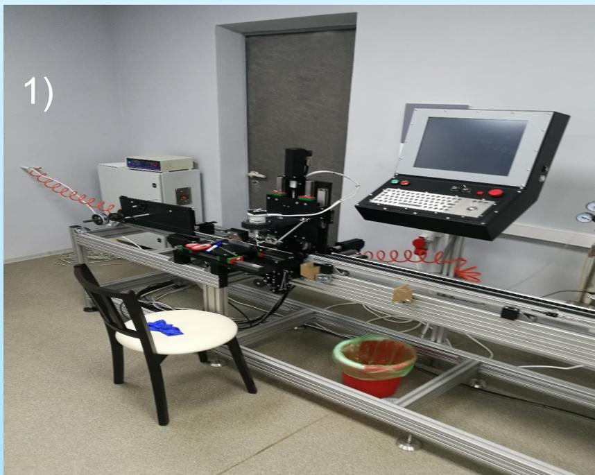
1) High Precision Ultrasonic Welding Machine, for the production of straws tubes
